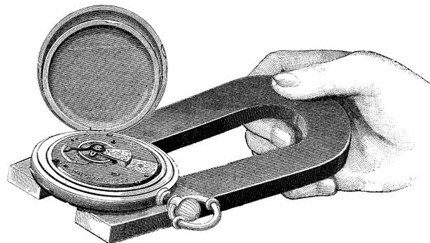
*Hermele movement and new style balance wheel, it was so magnetized that the clock would not regulate. After changing out the balance unit for an unmagnetized one I discovered that in addition virtually all the steel in this movement was magnetized as well. I finally found a very large TV degausser that worked and the movement regulated to 9000 BPH as required. The compass test is an important one.☺*
