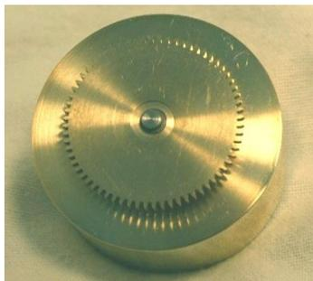
New main wheel attached to reconditioned barrel.
