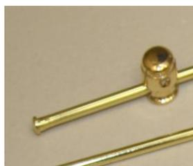
and center drilled, then tapped with a small tap such as a 1-72 or possibly a 2-56. A new “dimple” is fabricated with a threaded tail much like a screw but with no slot in the head,
