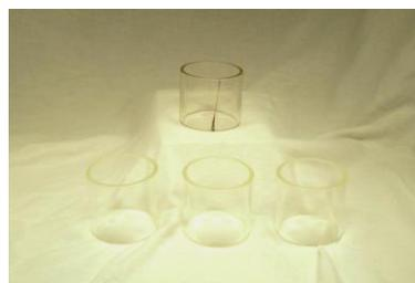
**Glass Sleeves.** Shown in the foreground are three cut sections of glass sleeve to be used as Spider cases.
