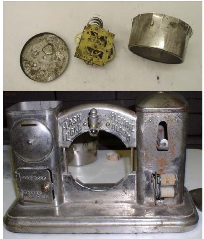
The basic idea behind the Darche Flashlight clock is fairly simple. The alarm key is replaced by a winding lever which, when the clock alarm activates, turns and causes contact with an electrically "hot" C shaped bar, closing the alarm circuit which activates the electric bell.
