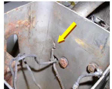
After either drilling out or removing the rivets holding the base of the "bank" unit internal to the left silo, the door and all buzzer rivets and coil yokes, the unit was disassembled into its parts and the restoration could finally begin.
