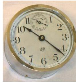
and protrusion from the dial required substantial trial and error. The result is shown to the left. Clearance to the hour hand was critical. Another point about the movement: a stop pin needed to be added near the center wheel pinion. This pin was not in the original design. Without it, the mainspring would impinge on the center wheel, stopping the clock long before it was unwound.
