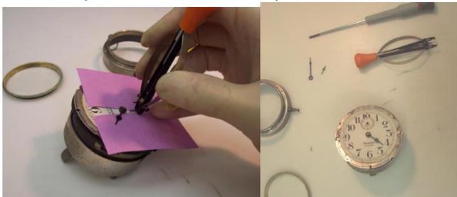
On the right is a view of the dial with hand safely removed as well as another view of the puller. No damage was done to the dial with this approach.
