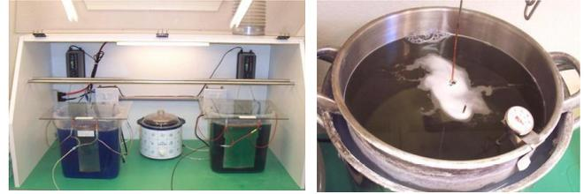
After cleaning and rinsing, into the copper tank it goes. The copper is a special EPI product that allows us to plate directly to steel without cyanide. Acid copper would corrode steel and could never plate it. The EPI product also has outstanding resistance to heat, which will serve well as we move forward in the restoration. On the right is the result.
