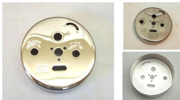
Here you see the completed rear bell, nickel plated. Lower inset is the inside view, also fully restored. Upper right inset is the "polished before" for comparison.
