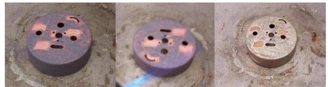
The middle picture is a little blurry, which is what happens when you try to take a picture with camera in your right hand, holding a hot blow torch in your left. On the right is the soldered surface.
