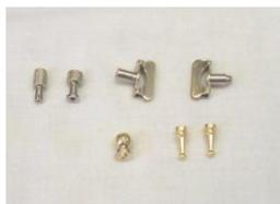
the top finial (loop) to accept a 2.0mm screw as shown here. All finials, setters and keys are then ultrasonically cleaned and
