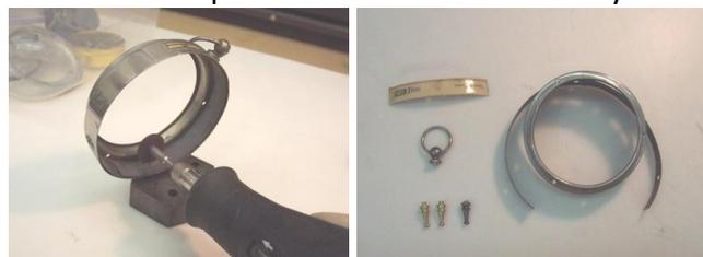
Not much repair work can be done to the front bezel until the nickel is removed. The nickel is a very tough barrier and impedes any smoothing or reshaping that must be done. Using our MetalX nickel stripper, the nickel is removed.
