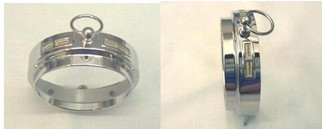
Following the assembly of the front bezel, the screws are reconditioned and plated. This is testimony to attention to detail. If the clock case is reconditioned and replated, the screws must also be reconditioned as well or they will look horribly out of place and detract from the quality of the restoration. Restoring the tiny screws can be time consuming since each one must be filed, reslotted, and finished as shown, then replated.
