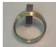
Working with Style 1 Baby Ben bezels can be a challenge because they are in the 0.012” thickness range. Style 1 and 1a Big Ben front bezels are much more workable at 0.018” or more, especially the earlier steel Style 1 Big Ben bezels. For the Style 1 Baby Ben bezels, it is possible to be too aggressive in sanding out nicks and scratches from the soft brass and sand right
