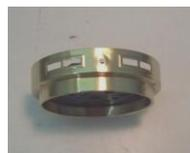
Why not use the pressure blasting approach? The blasting willpeen the thin brass which makes it very difficult to buff
