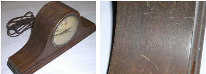
The right picture above is a close up of the finish. It can be seen that the finish has heavily alligatored. It is distressed, scratched, etc., but the real issue is the finish is failing. It will not easily dissolve because it has become dry and brittle. It cannot be partially removed because this process will continue to reveal more cracked and alligator effect underneath, all the way down to the bare wood. I will choose to remove it completely down to the bare wood.
