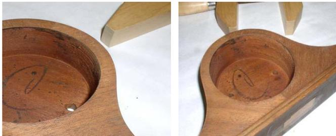
Once you have removed the clamps, you must do some minor touch up sanding around the edges of the veneer and over the surface to remove any excess glue that may have oozed out onto the surface. This also tends to blend the veneer patch to the surrounding area. Once you do this, you will have a finished result that looks as shown above. The repair is virtually invisible.
