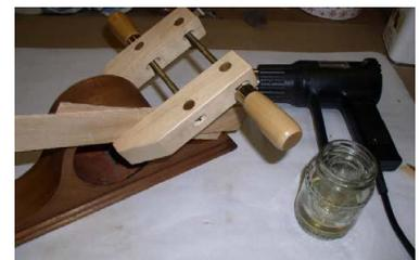
don't want to scorch the wood. But you want it warm in preparation for applying the glue. Apply the glue with a stick or toothpick to the clock case first, then to the veneer piece. You only need a thin coat of glue, not a heavy blob. Position the veneer in place and close the seam as best you can. Clean off any excess from the seam. Once the glue begins to get tacky (it will take only a minute or two for this to happen), confirm the
