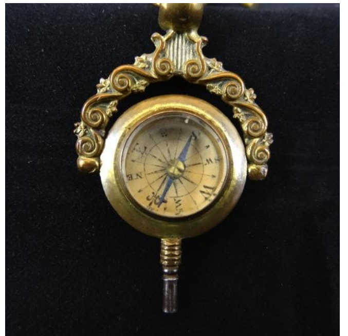
This key served a dual purpose: to wind your watch and to provide the direction.
