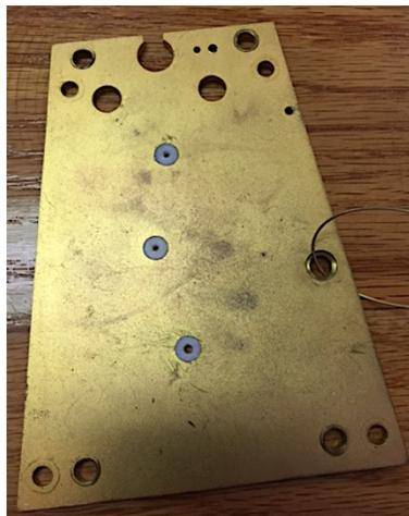
The pictures above show the plastic bushings, as well as a close up of one of the holes and the bushing that was removed. In researching these bushings, Dulen found that people cite several reasons to try to justify using these bushings including a self-lubricating design, corrosion and chemical resistance, superior longevity and wear.
